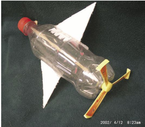
Fig. 5. AUV model made from pop bottle, toy propeller, and rubber bands. White wings are fins that stabilize the model and keep it from rotating as it swims. Designed by Dr. Patterson's graduate student, Lawrence Carpenter.
