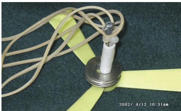
Fig. 6. Detail of toy prop. We removed the ring that connected the blade tops, using a pair of scissors. Note the washers on the end, which served as bearings (and affect the buoyancy), and the rubber bands tied to the end of the prop shaft that came off the toy.
